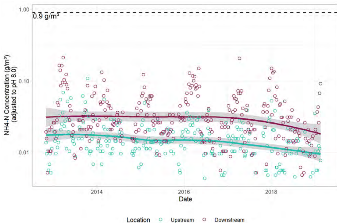
Figure 3: Ammonia concentration (total ammoniacal-N) adjusted to pH 8.0 (note the log scale on the y-axis). The lines of best fit through each location is a Loess fit and the shaded area is the 95% confidence interval of each fit. The dashed line is the ammonia toxicity standard from the PSWLP at pH 8.0.
