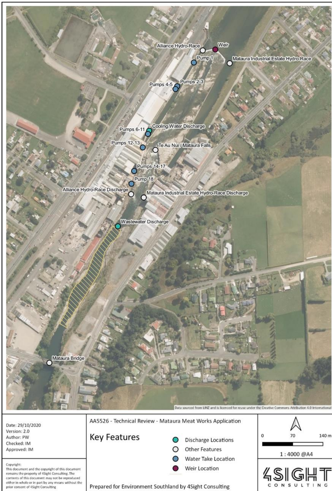
Figure 1: Aerial photograph of the Plant and key features
