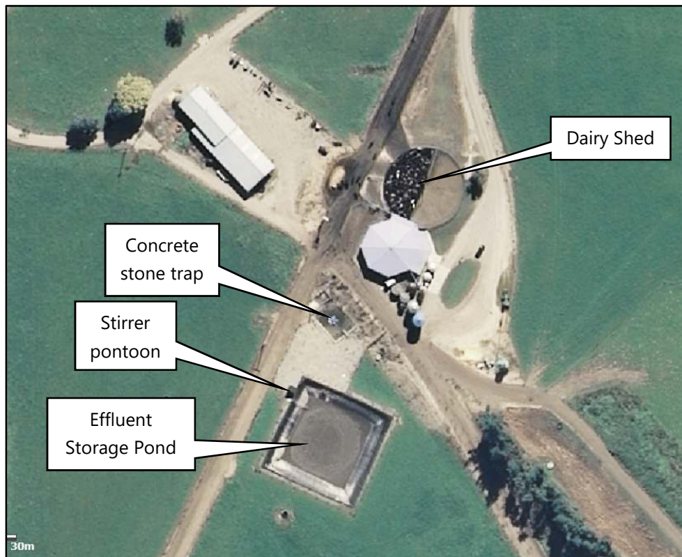
Figure 3: Overview of layout showing dairy shed and effluent treatment system (Source: ES Beacon, 2018).
