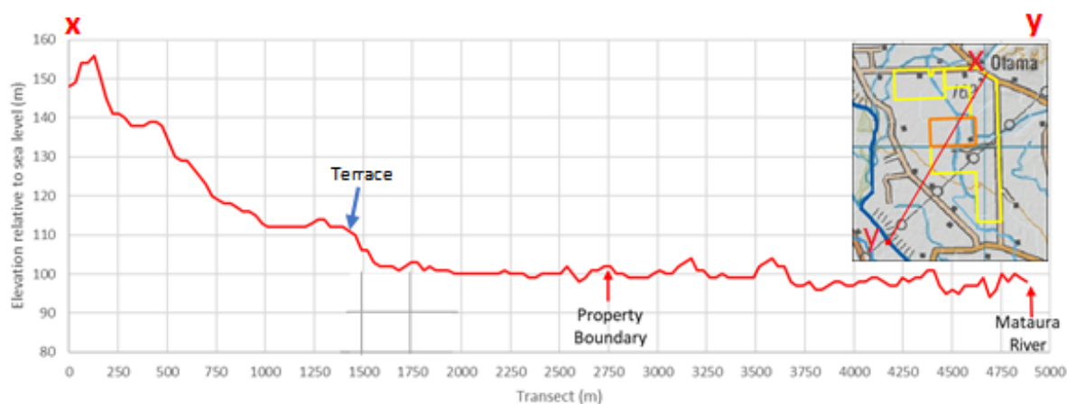
Figure 3: Transect across Cashmere Bay Dairy and Sheep Block (NASA Radar Topography). Otama (left) to Matura River (Right). Existing milking platform is shown in yellow and the sheep block in orange.
