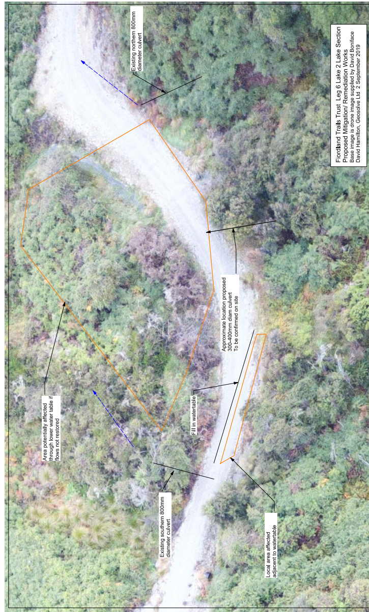
Figure 1: Drone image of section of trail showing proposed remediation work
