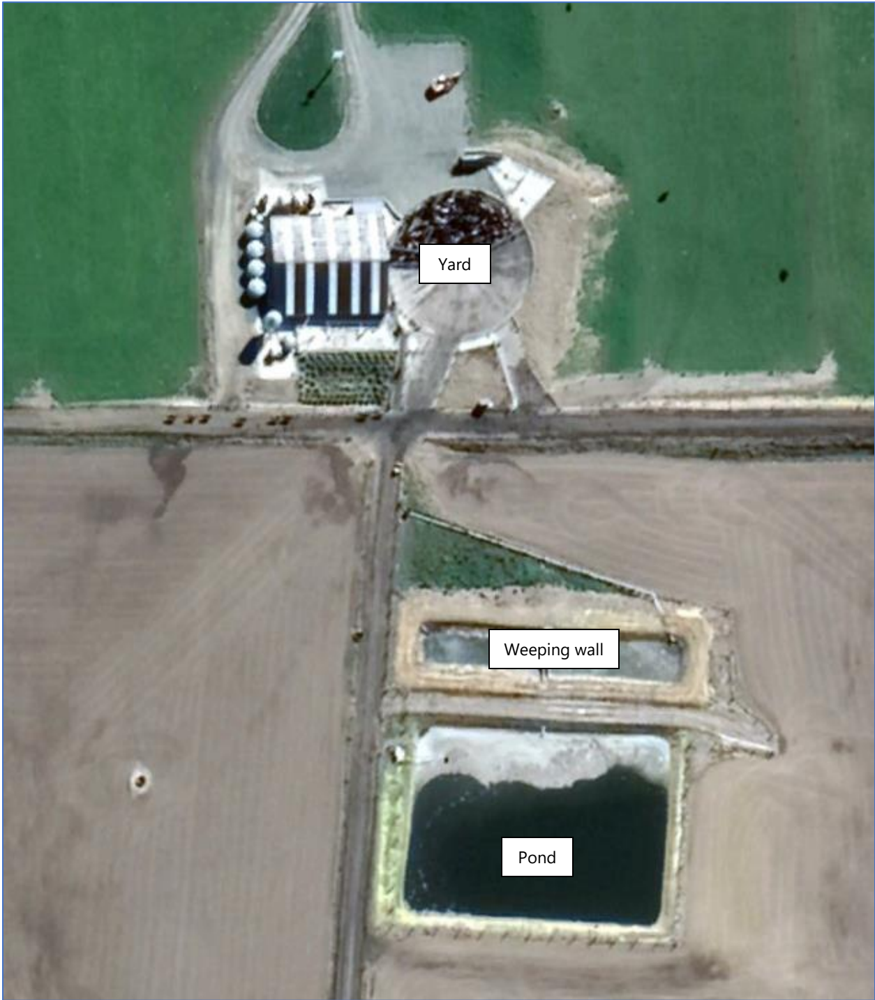
Figure 2: Effluent Infrastructure Layout
