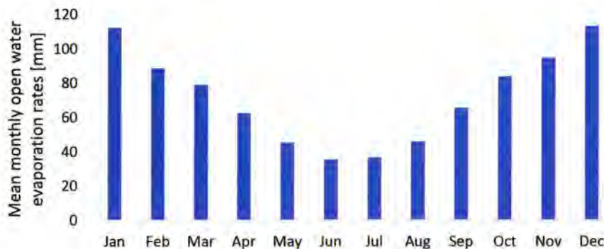
Figure 7: Mean monthly open water evaporation rates (Penman) in Invercargill using data from 1997 to 2018.
