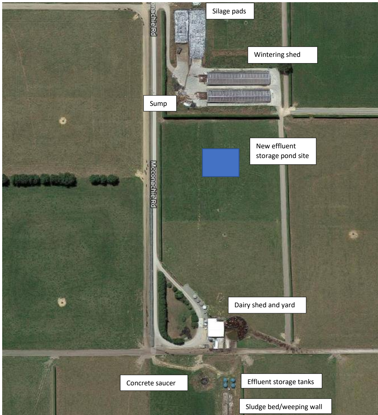
Figure 10: South Dairy 2 effluent system overview
