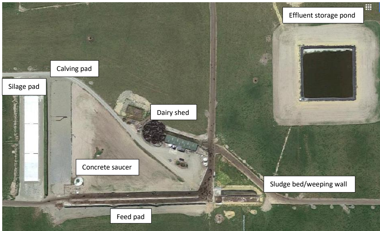
Figure 6: South Dairy 1 effluent system overview
