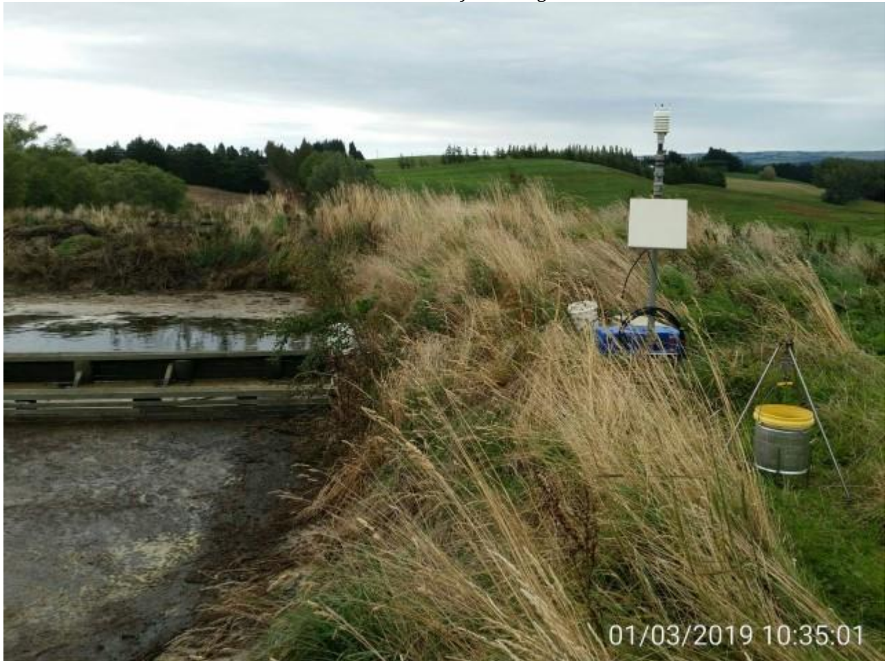
Laser at the south side of the sludge beds.
