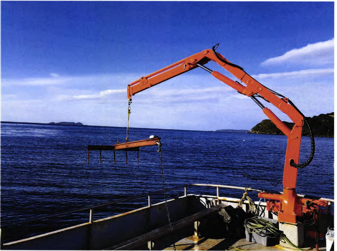
Photo 13: One of the anchors for a line of buoys being lifted onto the Stingray.
