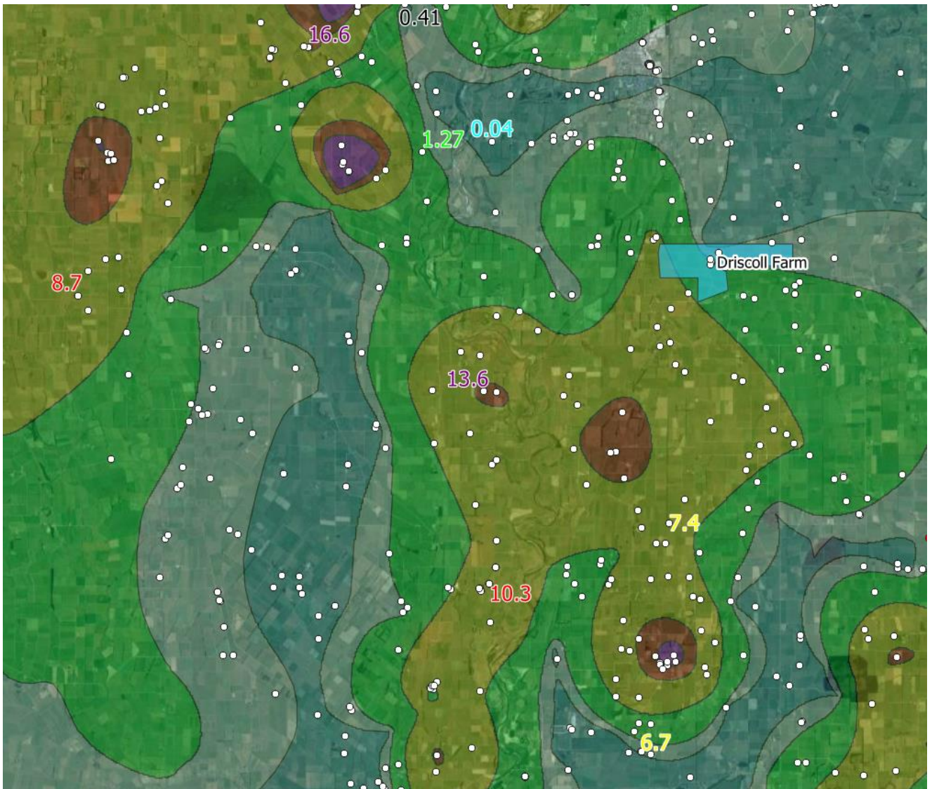
Figure 9 Peak nitrate N concentrations for groundwater from bores in the general area, post-2012 overlaid onto the 2007-2012 nitrate N concentration contour estimates
