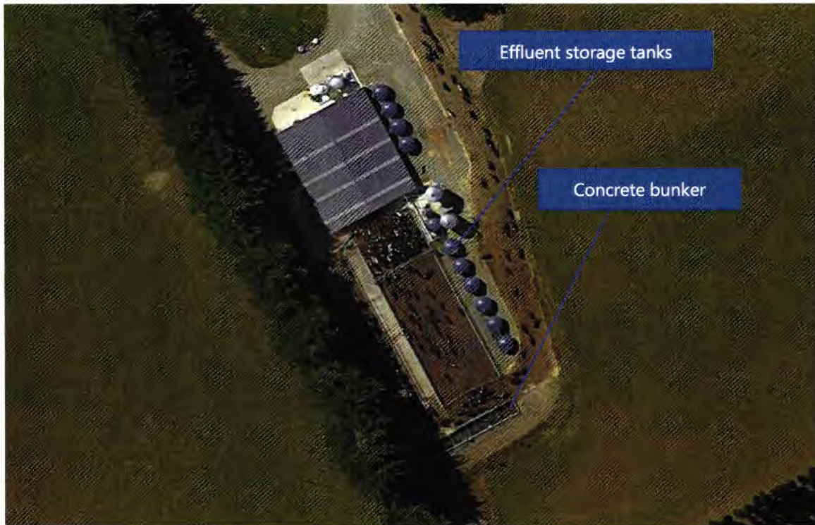
Figure 23: Layout plan of existing effluent storage facilities
