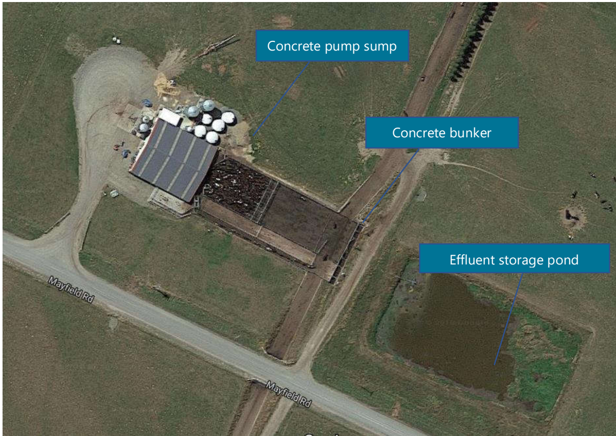
Figure 18: Layout plan of effluent storage facilities
