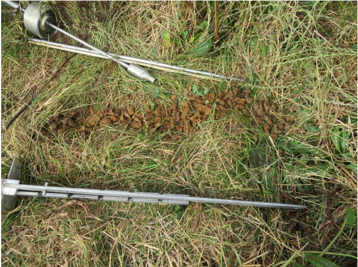
Figure 1. Photograph of Scala Penetrometer and material from auger hole.
