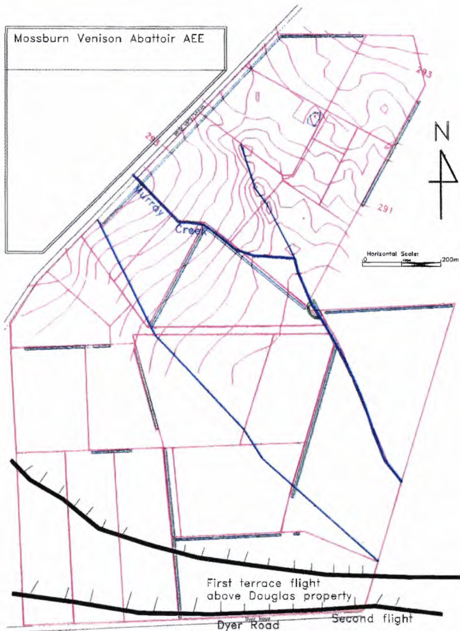
Figure 5.2 Contoured ground elevation in Deer Block and proximal sheep paddocks. Elevation is referenced to mean sea level. Main metre contours are marked.
