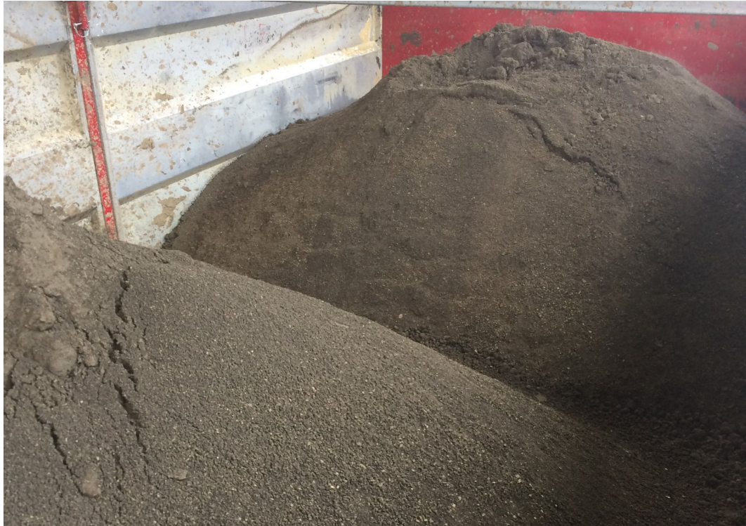
Figure 8: Final dried DAF solids ready to be taken off-site for composting.
