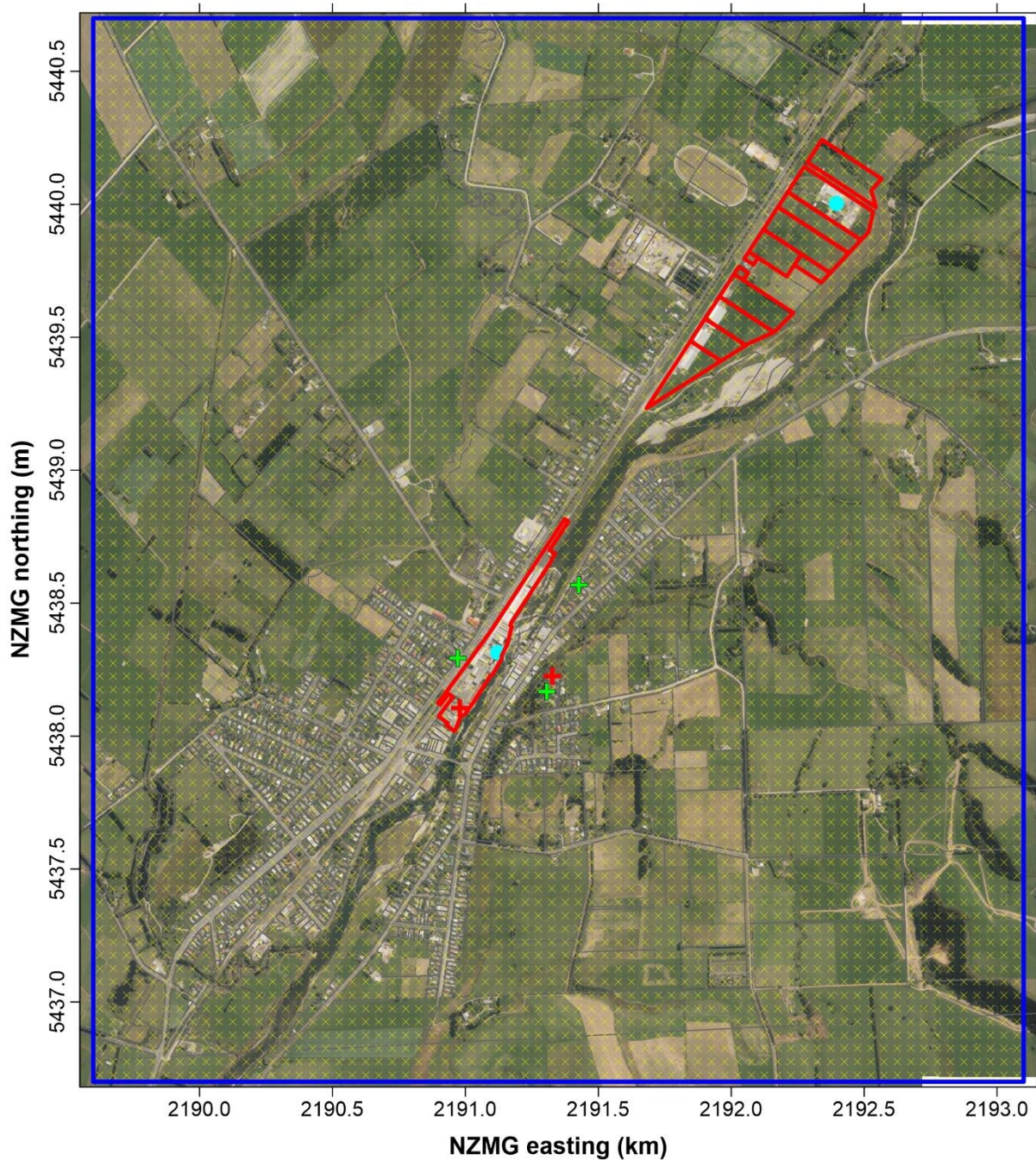
Figure 1: CALPUFF model domain. Sampling grids locations marked as yellow crosses, sensitive receptor locations marked as green crosses, monitoring sites marked as red crosses, the site boundary marked in red.
