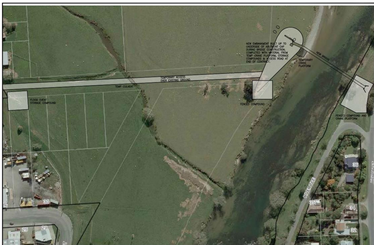
Figure 4: Fencing, access and storage locations during construction (Source: Concrete Structures Ltd, 2019, extract from Appendix C)
