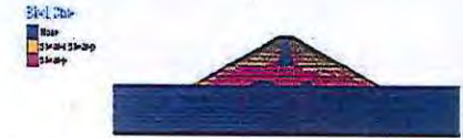
Fig. 7. Reference example: Distribution of plasticity in the dam (at maximum excitation). (-n: the zone is at active failure now; -p: the zone has failed in the past, shear, yield criterion -shear failure).
