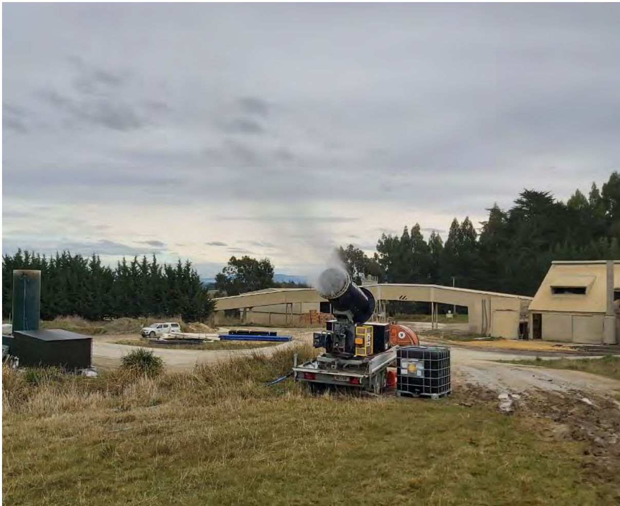
Figure 3. – Odour neutralising fog cannon.
