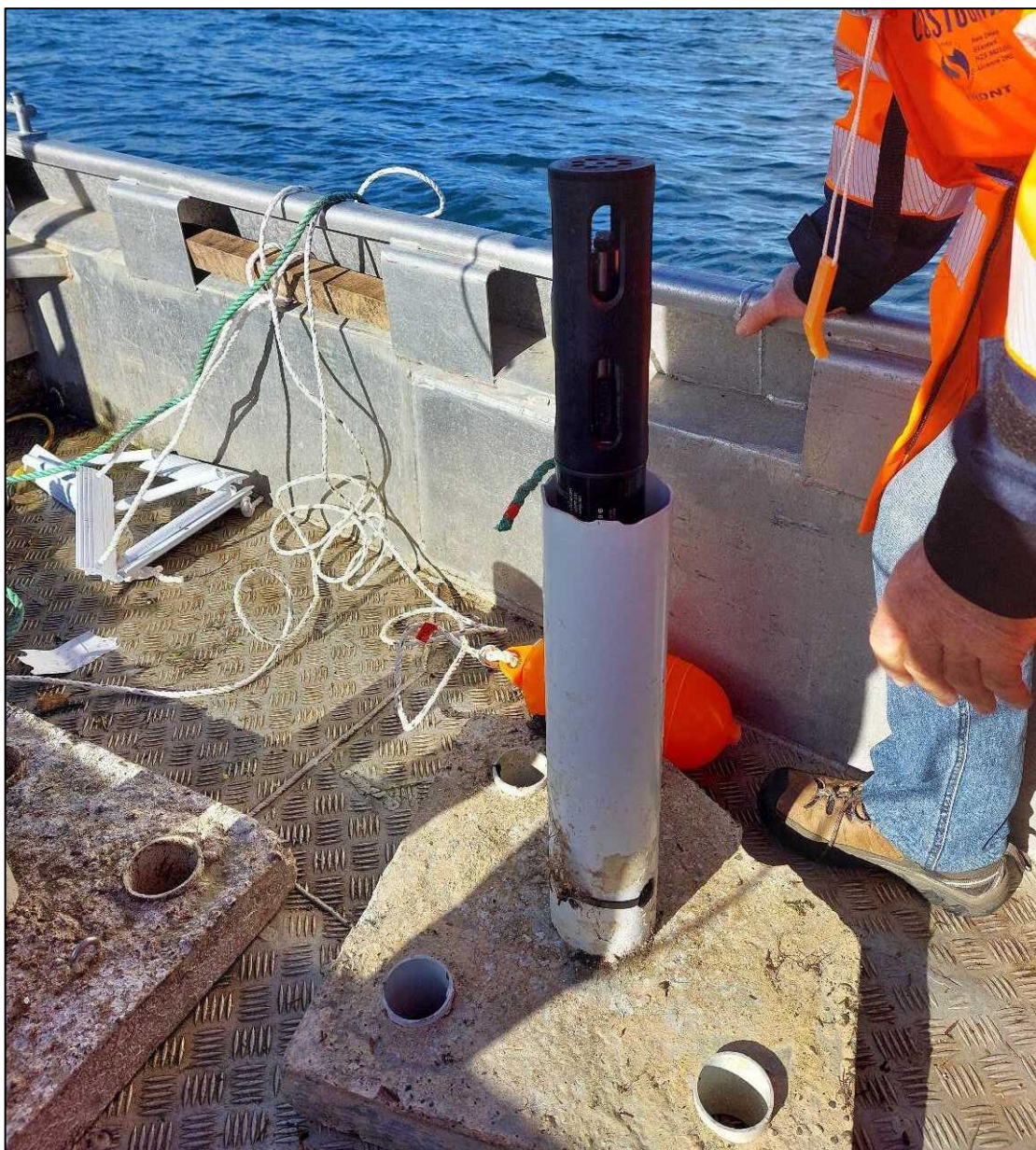
Figure 2: Turbidity logger deployment set-up.
