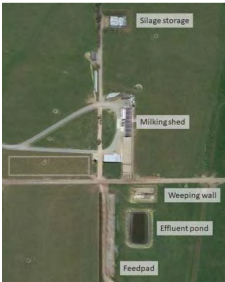
Figure 1: Details the proposed location of the new herd home winter barn and associated effluent storage bunker (grey rectangle to the west) in relation to the current dairy milking shed, feed pad and effluent system.
