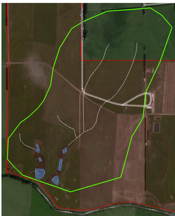
Figure 2. Schematic of the proposed wetland area (blue), the key tile drains that will be intercepted (white lines) and the catchment boundary (green). The farm boundary is shown by the red line. The total wetland catchment area is 44ha with 34ha of this falling within the property boundary.
