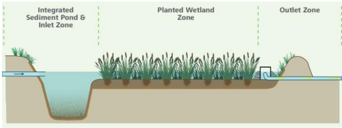
Figure 3. Schematic design of an integrated sediment pond and inlet zone style wetland (taken from Tanner et al. , 2022)
