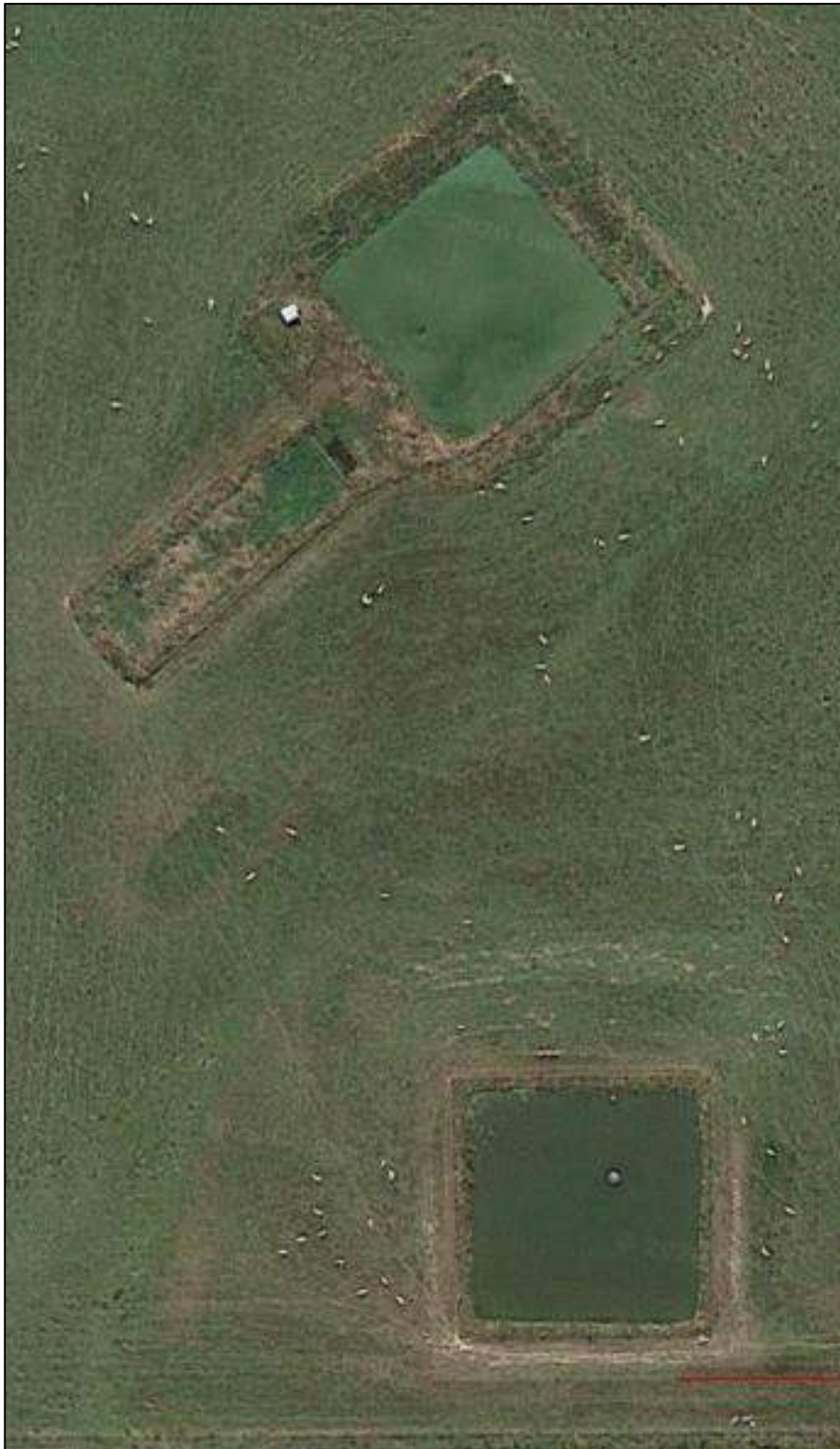
Figure 2.8: Aerial view of existing effluent ponds, weeping wall/sludge bed
