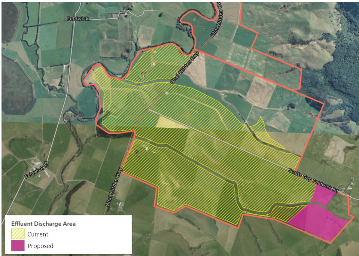
Figure 4: Effluent discharge area, 248.4ha, plus additional approx. 23 ha (pink), note buffers to be applied in this area.
