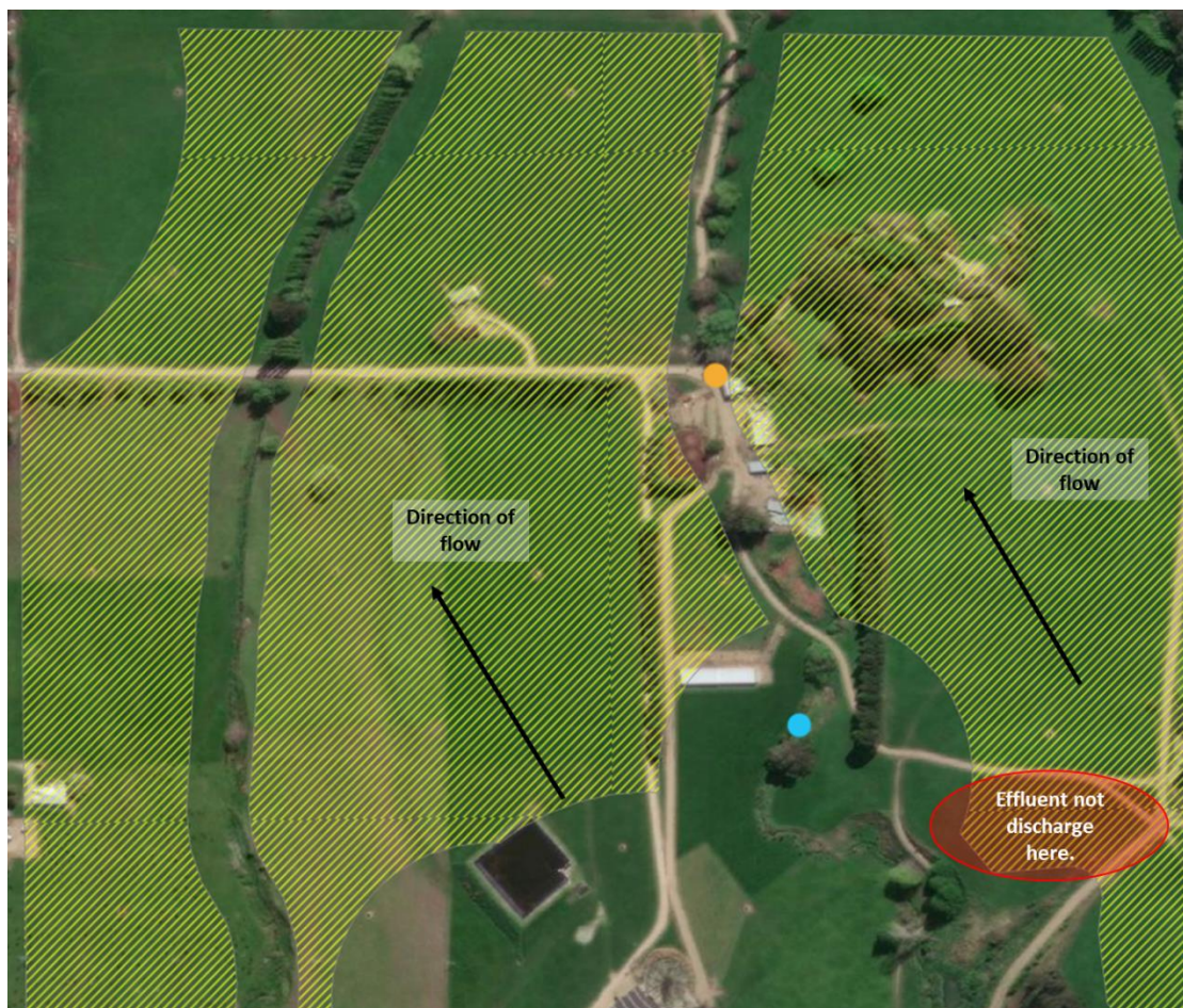
Figure 9: Location of GDC water abstraction point/pipe (blue) and pump shed (orange). Yellow is authorised discharge area.
