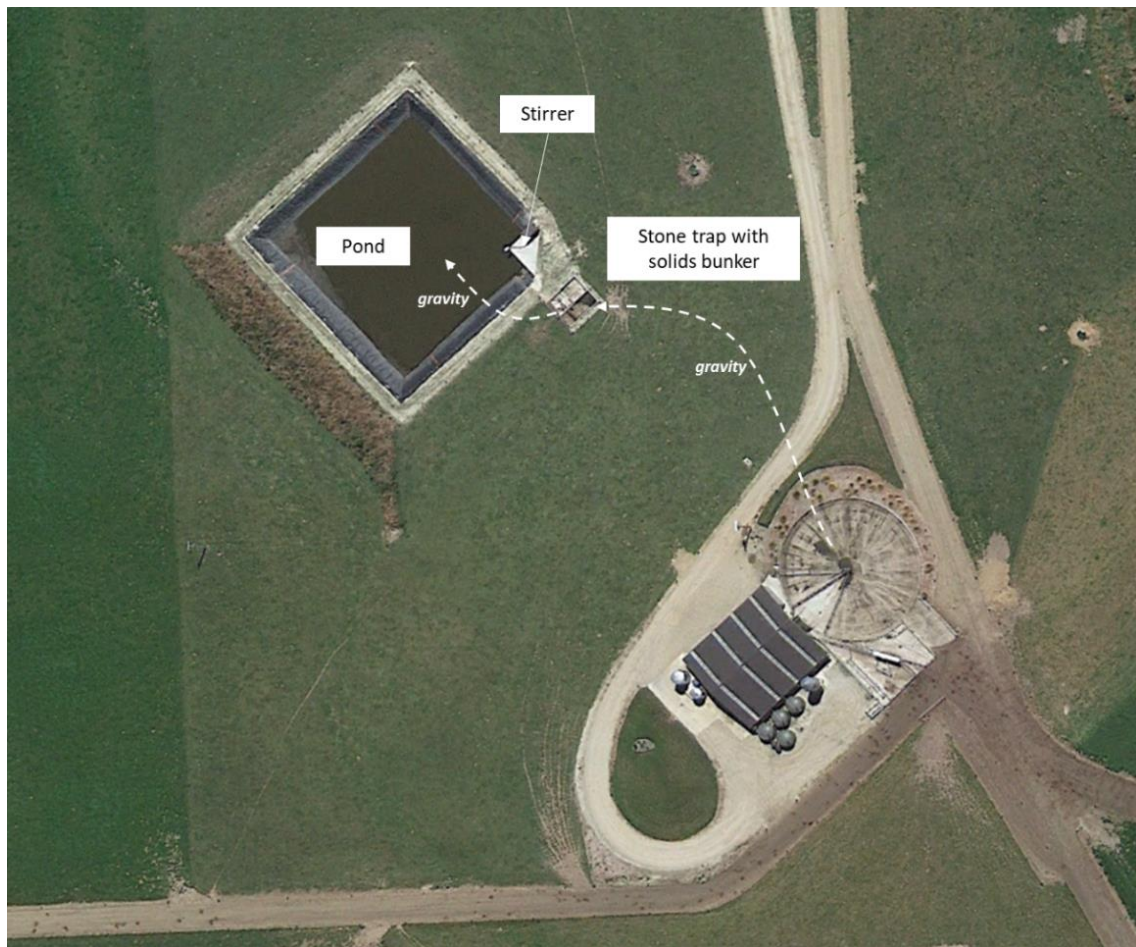
Figure 2: Effluent system overview.
