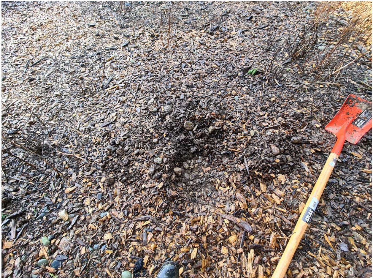
Figure 28 Pit dug showing compacted rock base.
