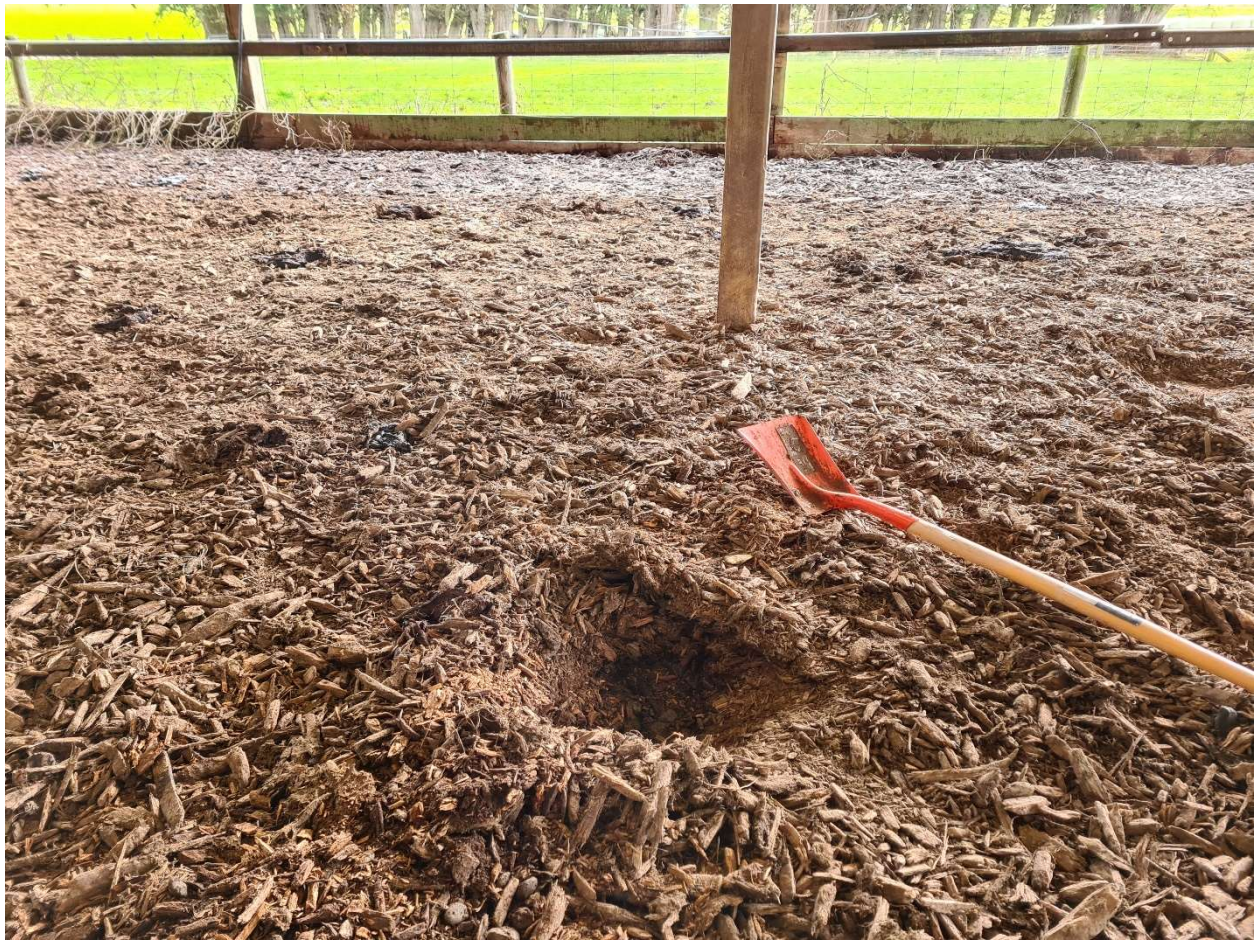
Figure 5 Pit dug in the south half of the roofed area showing layer of woodchip on top of a compacted rock base.
