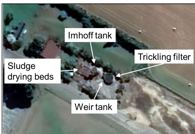
Figure 23 Balfour WWTP Layout
