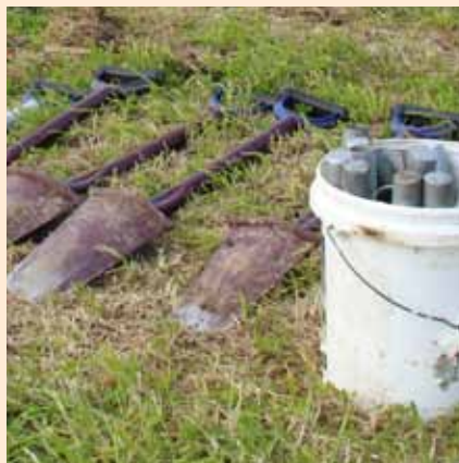
▲ We like to use tree-planting spades for digging and metal rammers to help push the stakes firmly into the ground. Buckets make the distribution of equipment to helpers easy and efficient.
