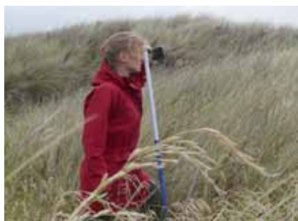
▲ The angle of the slope can be measured using a cell phone. (Download one of the free clinometer apps.)
