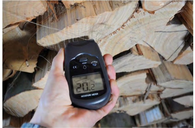
A moisture meter helps determine how dry your firewood really is.
