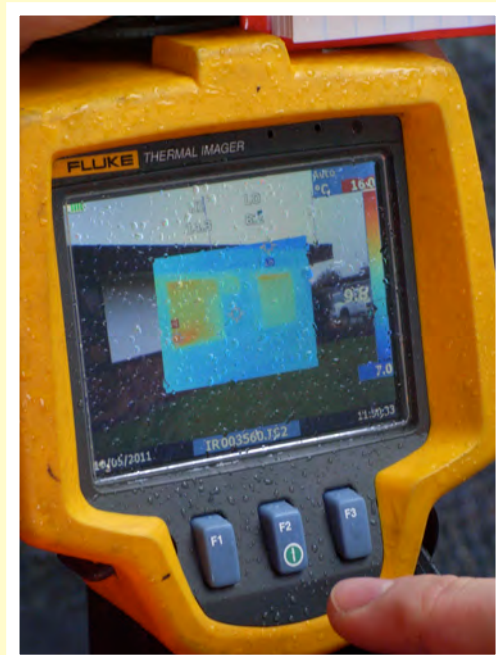
A thermal imaging camera can be used to detect heat leakage from a building.
