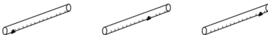
Clarity tube (note the magnet is moved from one end of the tube towards the other)
