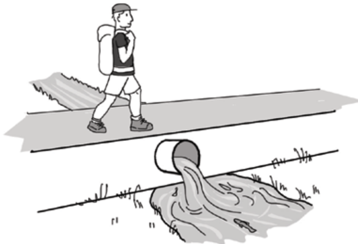
Poorly-designed culvert preventing fish passage upstream
