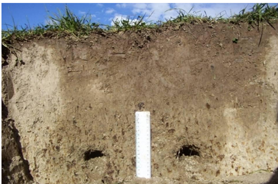
Figure 6. Field example of preferential flow through a Pallic soil containing remnants of old mole drains.
