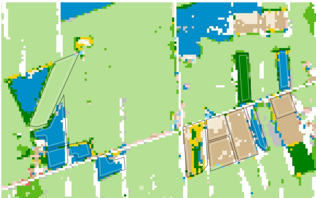
Figure 6 Accuracy assessment polygons overlaid on a very small section of the classification result. Environment Southland’s original polygons are displayed in black, with the buffered versions in white. The number of pixels in each class can be counted for each polygon, using Erdas Imagine’s ‘Summary’ function. The full classification result, along with its legend, is presented in the Results section.
