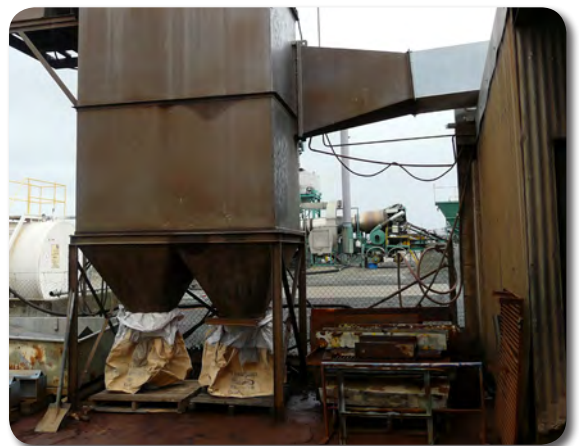
Steel blasting material is collected in bags for filtering and reuse.
