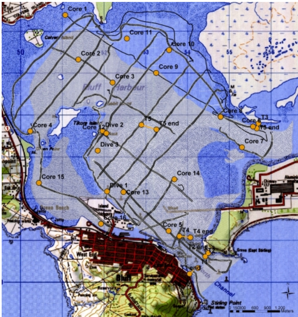
Figure 1 Bluff Harbour showing dive locations and side-scan sonar tracks, and the boundary of the subtidal area mapped (shaded area).
