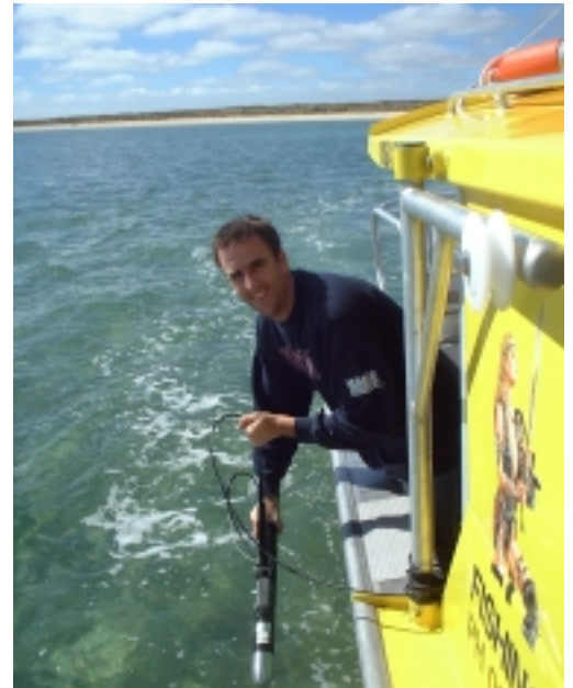
Figure 2 Deploying the sonar fish.
