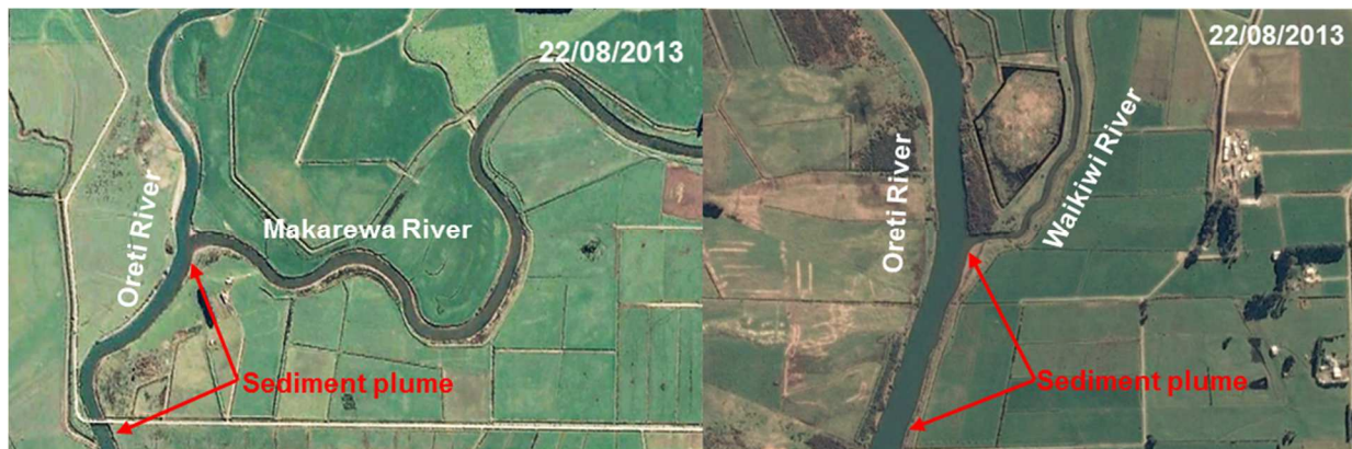
Figure 12: Sediment plumes from the Makarewa and Waikiwi Rivers cling to the shore on the true left bank of the Oreti River rather than mixing through the whole river below each confluence. [Google Earth images flown 22/08/2013].
