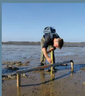
Measuring sediment depth: New River Estuary
