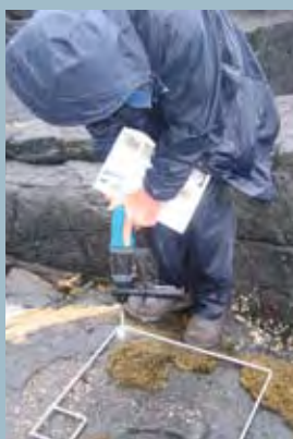
Figure 4. Fixed quadrat position markers - stainless steel bolts drilled into bedrock.
