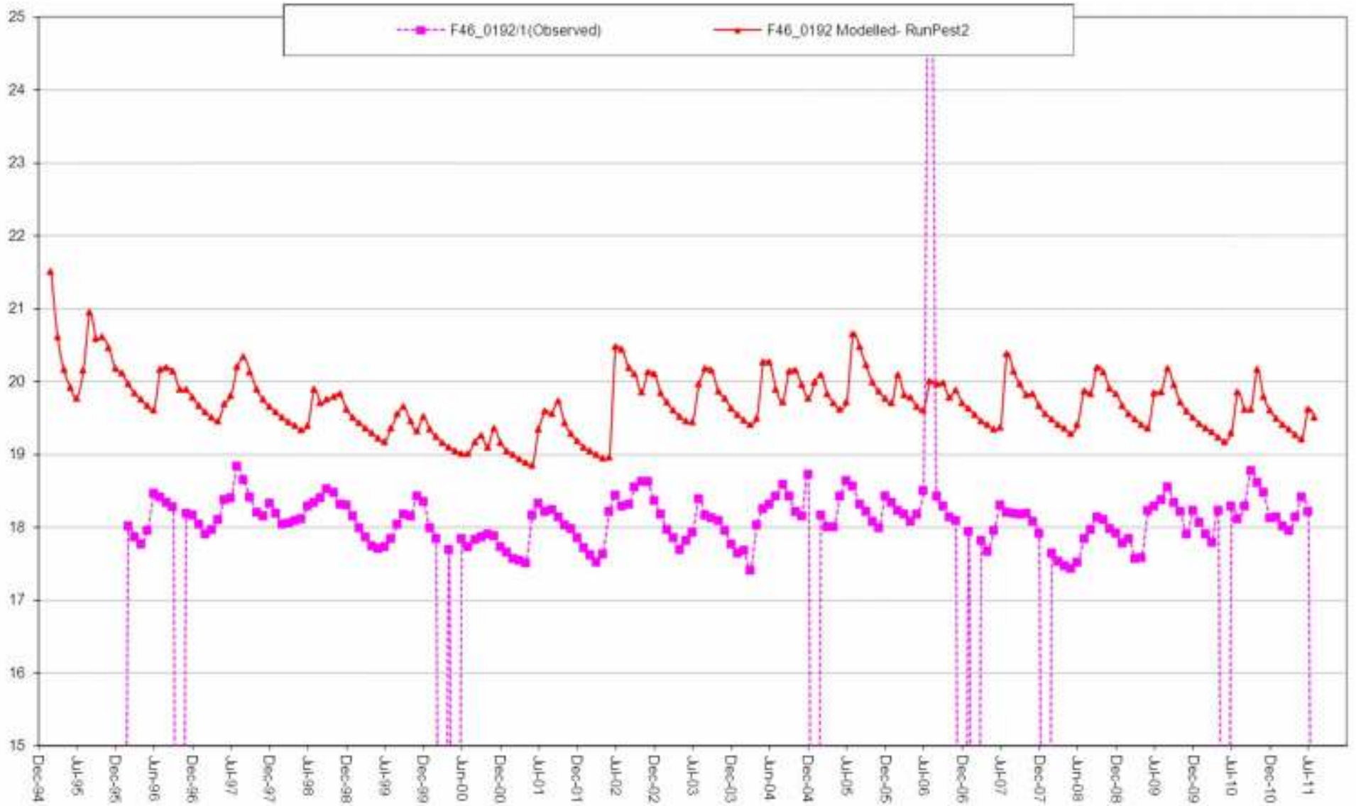
Figure 5e: Modelled and Observed Groundwater Hydrograph for F46/0192
