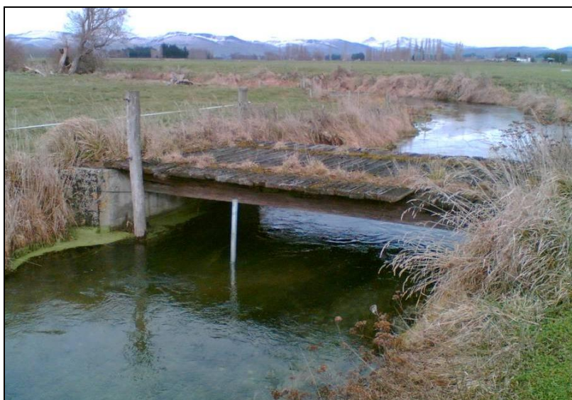
Figure 16: Photograph of the Meadow Burn 500 metres downstream of Fingerpost Pyramid Road with in-stream piezometer [source: K Wilson, 21 st June 2006]
