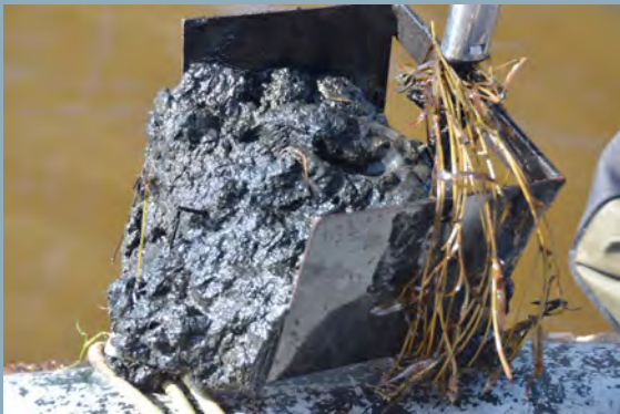
Sulphide rich sediments on the bed of The Reservoir at western end, February 2013.
